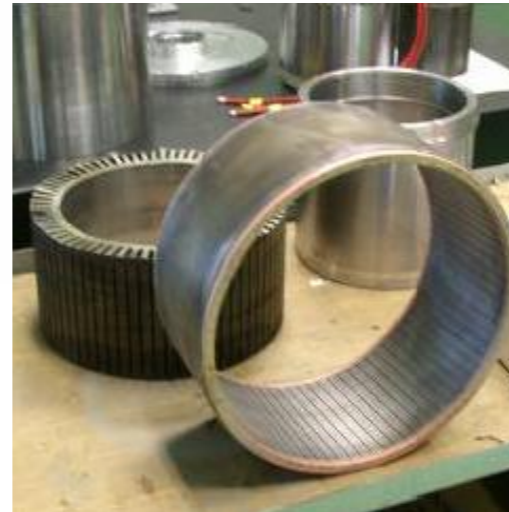
Outer rotor, high torque induction machine
