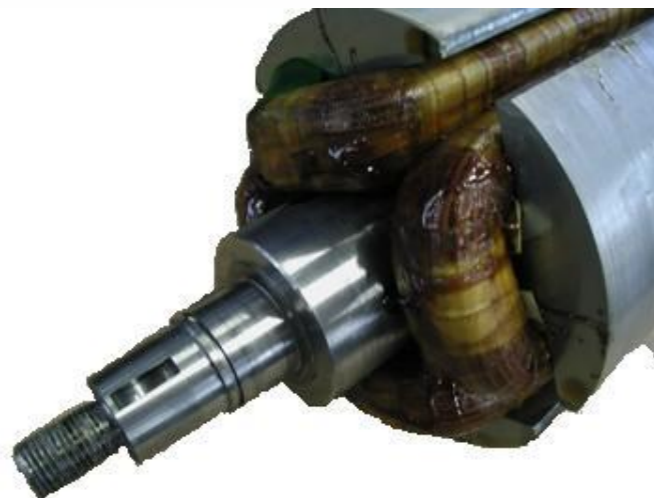
WR-SM wound rotor synchronous machine
